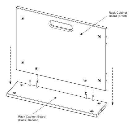
Lay the second rack cabinet back board down with cam pins and locks facing up. Slide front rack cabinet board onto the back rack cabinet board. Cam locks facing hardware on small board. Place screw driver into cam lock and turn clock wise to lock cam pins in place (2 Total)
