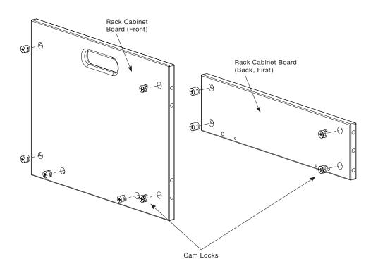
Push six cam locks into the front rack cabinet board.
