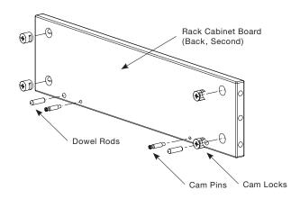
Use the second rack cabinet back board. Place dowel rods, cam pins, and cam locks into board. Cam locks go into the largest holes, dowel rods in the next size hole. Finally, cam pins go into the smallest holes and need to be screwed into the back board.
