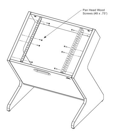
Stand the rack cabinet up and find the four inside pilot holes on each side. Attach rack rails with four pan head wood screws (#8 x .75") on each side. Install screws on the top, middle and bottom of rack rails.
