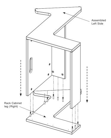
Lay the left rack cabinet leg down with the hardware facing up. Slide the first rack cabinet back board into the left rack cabinet leg. Make sure the cam locks are facing inside. Slide assembled front rack cabinet onto left rack cabinet leg. Place screw driver into cam locks and turn clock wise to lock cam pins in place (6 Total)
