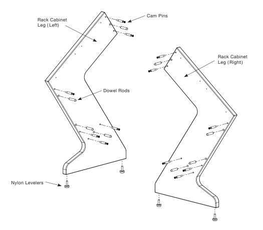
Screw in six cam pins and push four dowel rods into each of the side rack cabinet boards. Small holes are for the cam pins and the larger holes are for the dowel rods. Screw two nylon levelers into each of the rack cabinet board bottoms.
