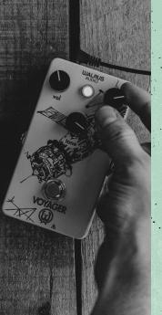
VOLUME - The Volume knob sets the overall output of the pedal.
